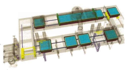
The transport system for manufacturing solar cells operates completely in vacuum. Products move from the Loadlock IN position to Loadlock OUT stopping at up to 18 process stations along the way.
